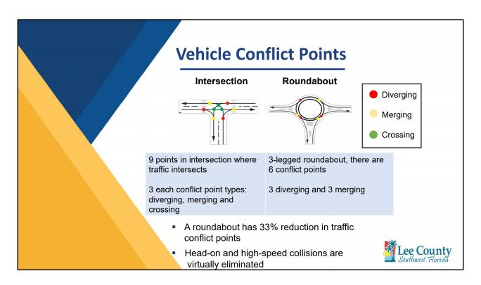
As it exists today, there are 9 points in the intersection where traffic intersects – 3 of each of the conflict point types: diverging, merging and crossing. In a three-legged roundabout, there are 6 conflict points – 3 diverging and 3 merging. In addition to a 33% reduction in traffic conflict points, head-on and high-speed collisions are virtually eliminated.
