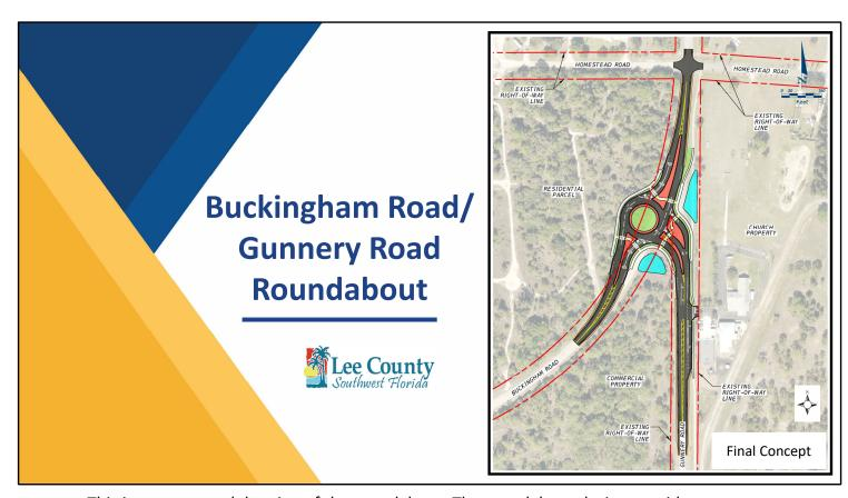
This is a conceptual drawing of the roundabout. The roundabout design provides a separate northbound right turn lane to Buckingham Road from Gunnery Road, and a separate southbound through lane along Buckingham Road. Right-of-way needs have not been confirmed or approved by the Board of Lee County Commissioners.
